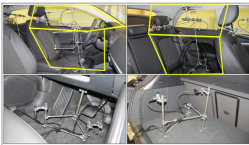
Figure 28. Microphones location for trimmed body measurements
